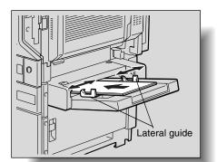
Push the lateral guides firmly up against the edges of the paper.
